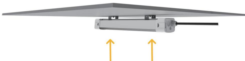
⑥ Fix the fitting to the mounting holder or suspension kit.
